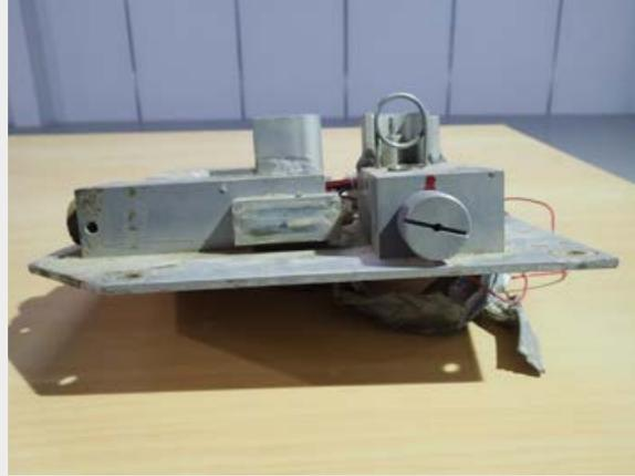
Wires from each of the four switches converge on the baseplate, where they are combined in a four-pin electrical plug socket. A four-pin plug connects a single, Simia-branded cable to the baseplate socket. This cable runs sternwards, below deck, to an improvised arming switch (Figure 9 and Schema 2, B). The switch consists of two spring-loaded
